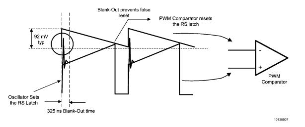
FIGURE 2. Basic Operation of the PWM Comparator
