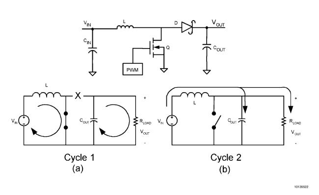
FIGURE 8. Simplified Boost Convertert A. First Cycle Operation B. Second Cycle of Operation
