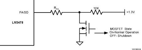
FIGURE 7. Shutdown Operation in Frequency Adjust Mode
