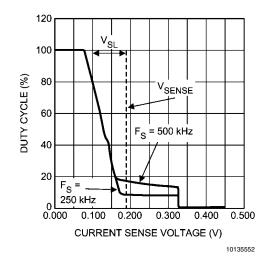
FIGURE 10. Current Sense Voltage vs Duty Cycle
