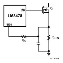
FIGURE 4. Adding External Slope Compensation
