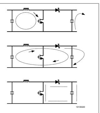
FIGURE 12. Current Flow In A Boost Application
