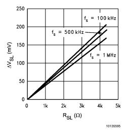
FIGURE 5. External Slope Compensation  $\Delta V_{SL}$  vs  $R_{SL}$
