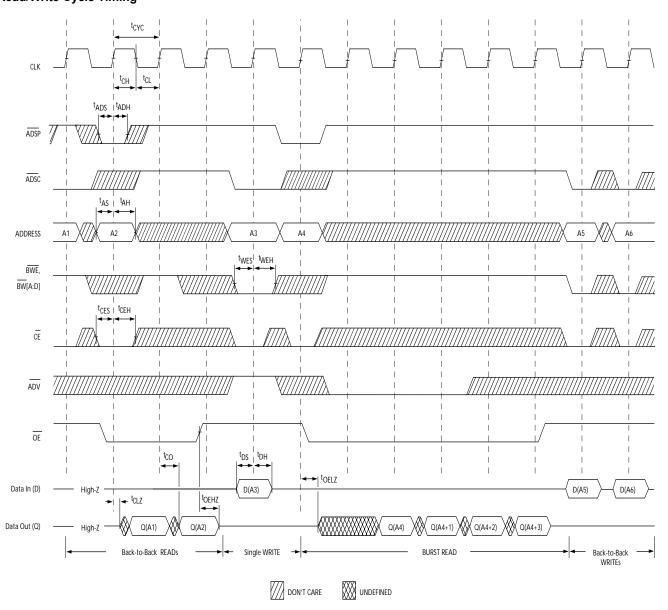
Note: 19. The data bus (Q)remains in high-Z following a WRITE cycle, unless a new read access is initiated by ADSP or ADSC. 20. GW is HIGH
