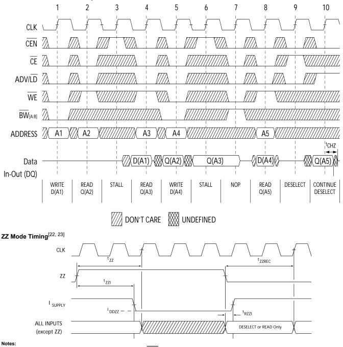
21. The IGNORE CLOCK EDGE or STALL cycle (Clock 3) illustrated CEN being used to create a pause. A write is not performed during this cycle. 22. Device must be deselected when entering ZZ mode. See cycle description table for all possible signal conditions to deselect the device. 23. DQs are in high-Z when exiting ZZ sleep mode.
