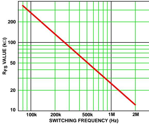
FIGURE 23. R_{FS} vs SWITCHING FREQUENCY
