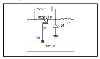
The RC components should realise a time constant corresponding to one tenth of the switching time constant of the TSM108 (i.e. in our example, the oscillator frequency is set to 10µs corresponding to 100kHz, therefore, the RC couple should realise a time constant close to 1µs).
