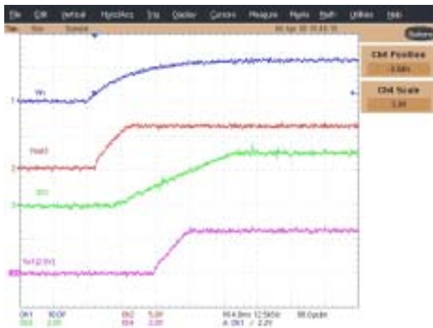
Figure 21 - Start up waveforms for 2.5V output Ch1: Vin, Ch2: Vout3, Ch3: SS1, Ch4: Vo1 (2.5V)
