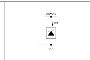
Figure 11. Test circuit for Vka > Vref
