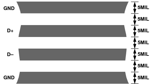
Figure 28. Arrangement of Signal Tracks
