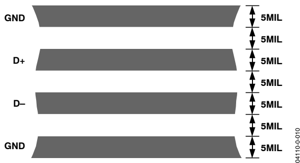
Figure 24. Typical Arrangement of Signal Tracks
