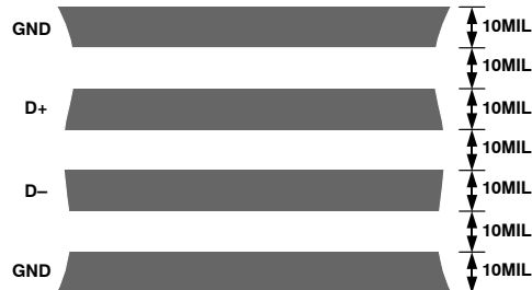
Figure 19. Arrangement of Signal Tracks
