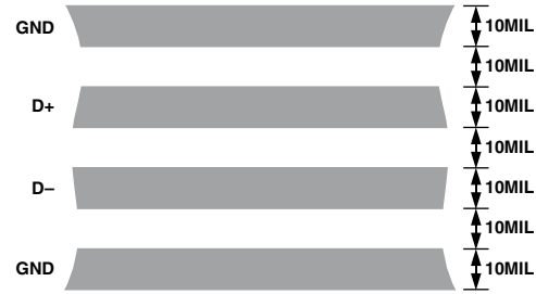
Figure 4. Arrangement of Signal Tracks
