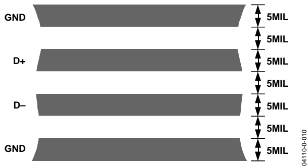
Figure 24. Typical Arrangement of Signal Tracks
