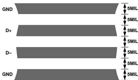
Figure 28. Arrangement of Signal Tracks
