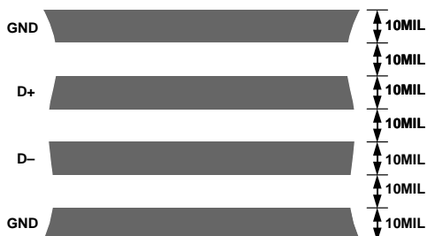
Figure 18. Arrangement of Signal Tracks
