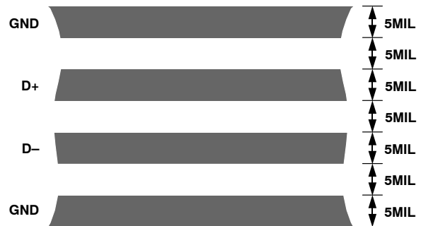
Figure 21. Typical Arrangement of Signal Tracks
