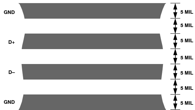
Figure 23. Typical Arrangement of Signal Tracks
