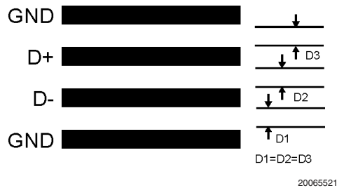
FIGURE 11. Ideal Diode Trace Layout
