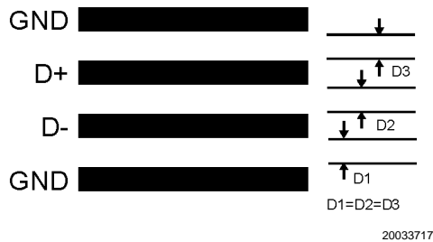
FIGURE 15. Ideal Diode Trace Layout
