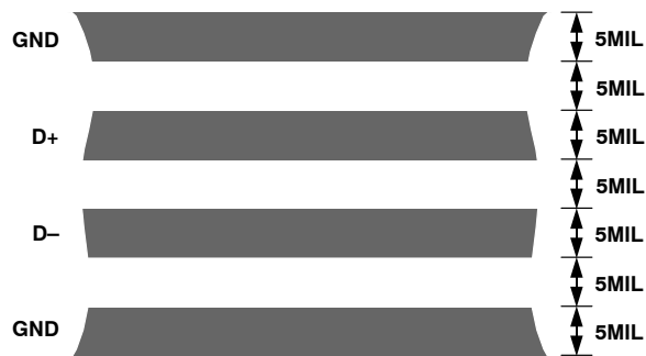
Figure 34. Typical Arrangement of Signal Tracks
