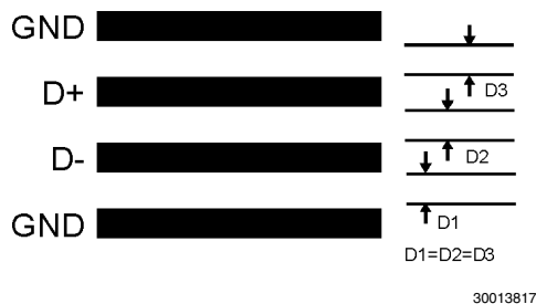
FIGURE 9. Ideal Diode Trace Layout
