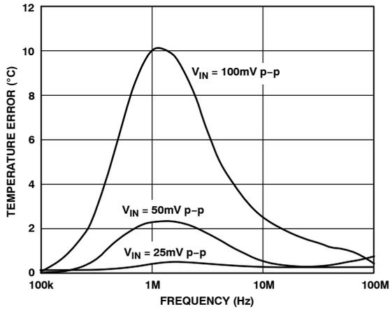
Figure 9. Temperature Error vs. Common-Mode Noise Frequency
