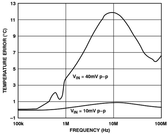
Figure 5. Temperature Error vs. Differential Mode Noise Frequency
