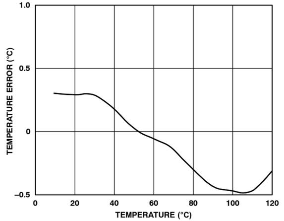
Figure 4. Temperature Error vs. Actual Temperature Using 2N3906
