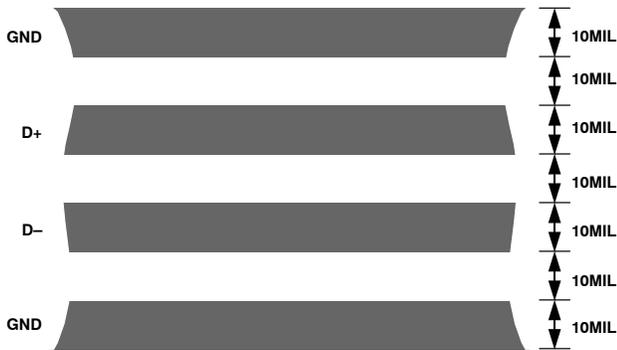
Figure 18. Typical Arrangement of Signal Tracks
