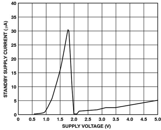
Figure 11. Standby Supply Current vs. Supply Voltage
