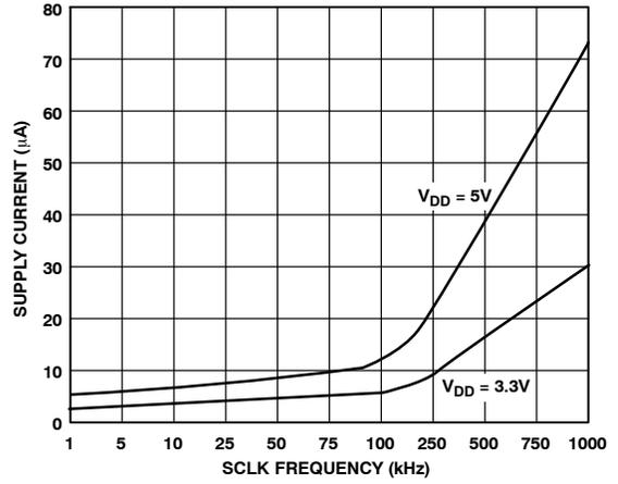
Figure 10. Standby Supply Current vs. Clock Frequency
