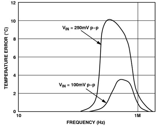
Figure 6. Temperature Error vs. Power Supply Noise Frequency
