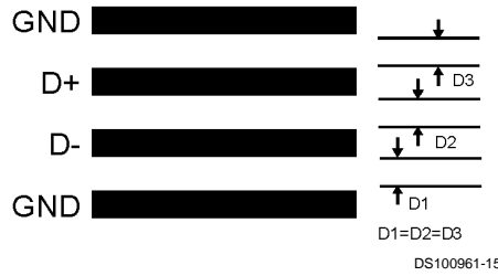
FIGURE 6. Recommended Diode Trace Layout
