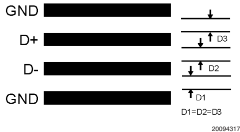
FIGURE 4. Ideal Diode Trace Layout
