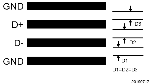
FIGURE 4. Ideal Diode Trace Layout
