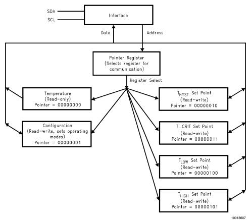
The data registers in the LM77 are selected by the Pointer register. At power-up the Pointer is set to "00"; the location for the Temperature Register. The Pointer register latches the last location it was set to. In Comparator Interrupt Mode, a read from the LM77 resets the INT output. Placing the device in Shutdown mode resets the INT and T\_CRIT\_A outputs. All registers are read and write, except the Temperature register which is read only.
