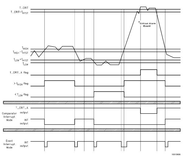
Note: Event Interrupt mode is drawn as if the user is reading the part. If the user doesn't read, the outputs would go low and stay that way until the LM77 is read.
