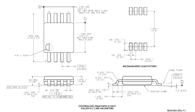
8-Lead (0.150 Wide) Molded Mini Small Outline Package (MSOP), JEDEC Registration Number MO-187 (variation AA), Order Number LM77CIMM-3, LM77CIMMX-3, LM77CIMM-5 or LM77CIMMX-5 NS Package Number MUA08A
