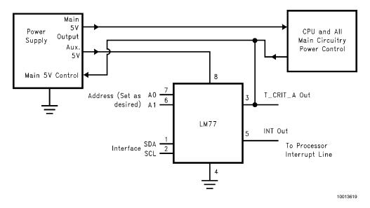
FIGURE 10. ACPI Compatible Terminal Alarm Shutdown. By powering the LM77 from auxiliary output of the power supply, a non-functioning overheated computer can be powered down to preserve as much of the system as possible.
