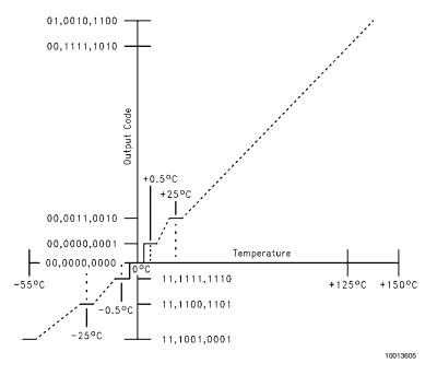
FIGURE 2. Temperature-to-Digital Transfer Function (Non-linear scale for clarity)
