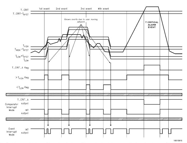
Note: Event Interrupt mode is drawn as if the user is reading the part. If the user doesn't read, the outputs would go low and stay that way until the LM77 is read.
