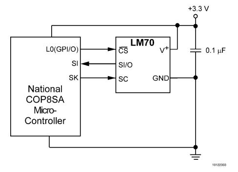
**FIGURE 1. COP Microcontroller Interface**
