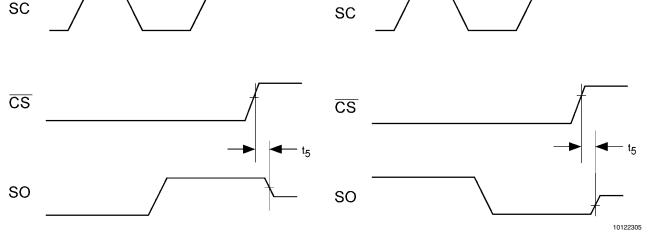
FIGURE 3. TRI-STATE Data Output Timing Diagram
