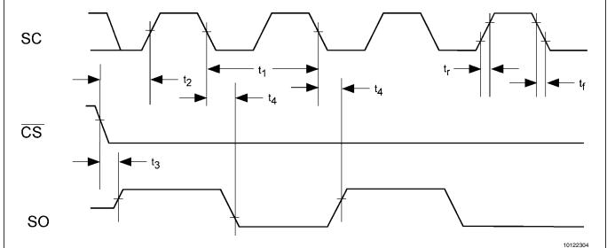
FIGURE 2. Data Output Timing Diagram
