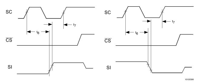
FIGURE 4. Data Input Timing Diagram
