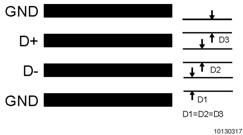
FIGURE 15. Ideal Diode Trace Layout
