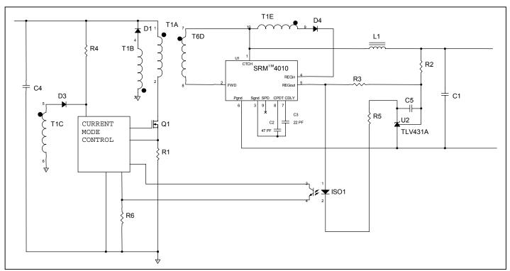
Figure 8 SRM<sup>TM</sup>4010 Configured for outputs below 1.25 Volts
