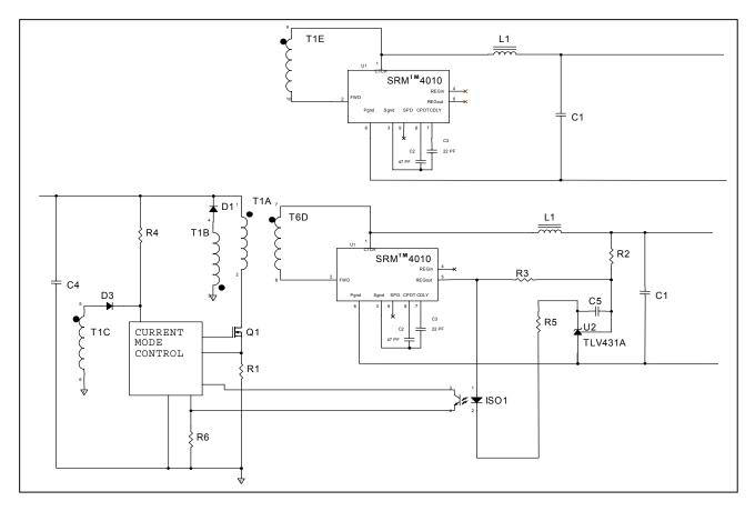
Figure 9 SRM<sup>TM</sup>4010 Multiple Output Configuration
