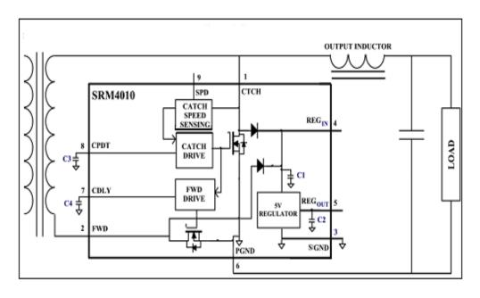
Figure 6 SRM<sup>TM</sup>4010 Forward Converter Block Diagram
