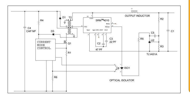
Figure 7 SRM<sup>TM</sup>4010 In a typical 1.25 To 3 Volt output Isolated Power Converter
