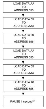
1. Data Format: I/O7 - I/O0 (Hex); Notes: Address Format: A14 - A0 (Hex). 2. Boot block lockout feature enabled.
