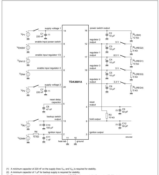
(3) These capacitors represent the typical input capacitance of CMOS logic connected to the reset and hold outputs.
