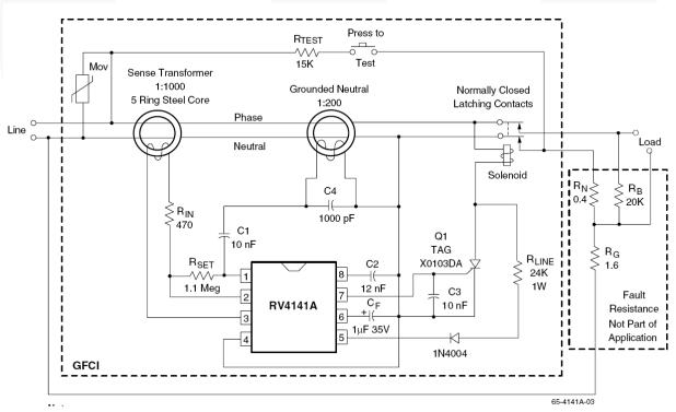
Figure 3. GFI Application Circuit
