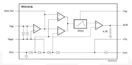
Figure 1. Block Diagram
