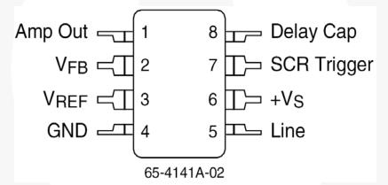
Figure 2. Pin Assignment
