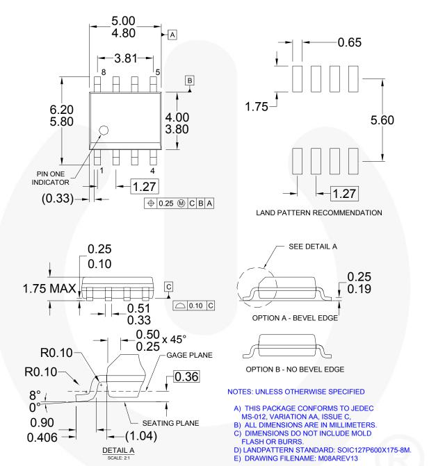
Figure 5. 8-Lead, Plastic Small-Outline Integrated Circuit (SOIC)
