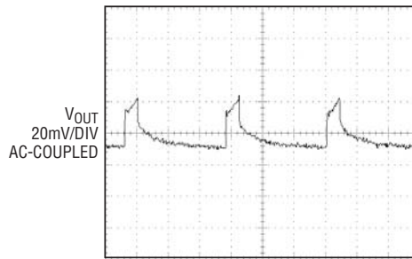
Output Voltage Waveform When V_{MID} is Shorted to V_{OUT}
