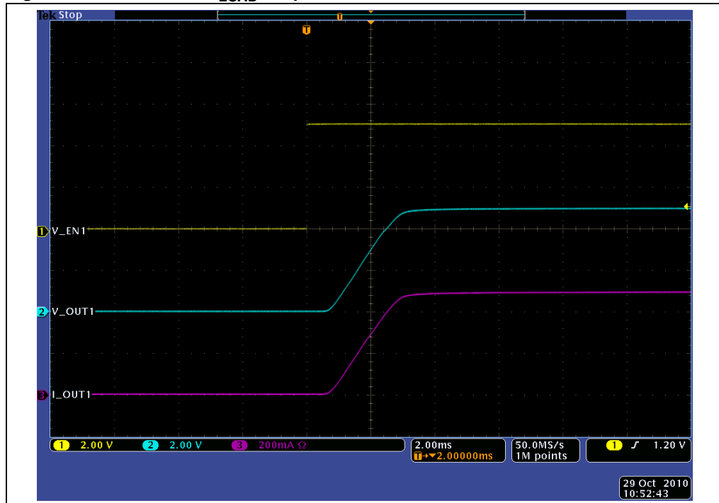
Figure 9. Turn-on for C_{LOAD} = 1 \mu F
