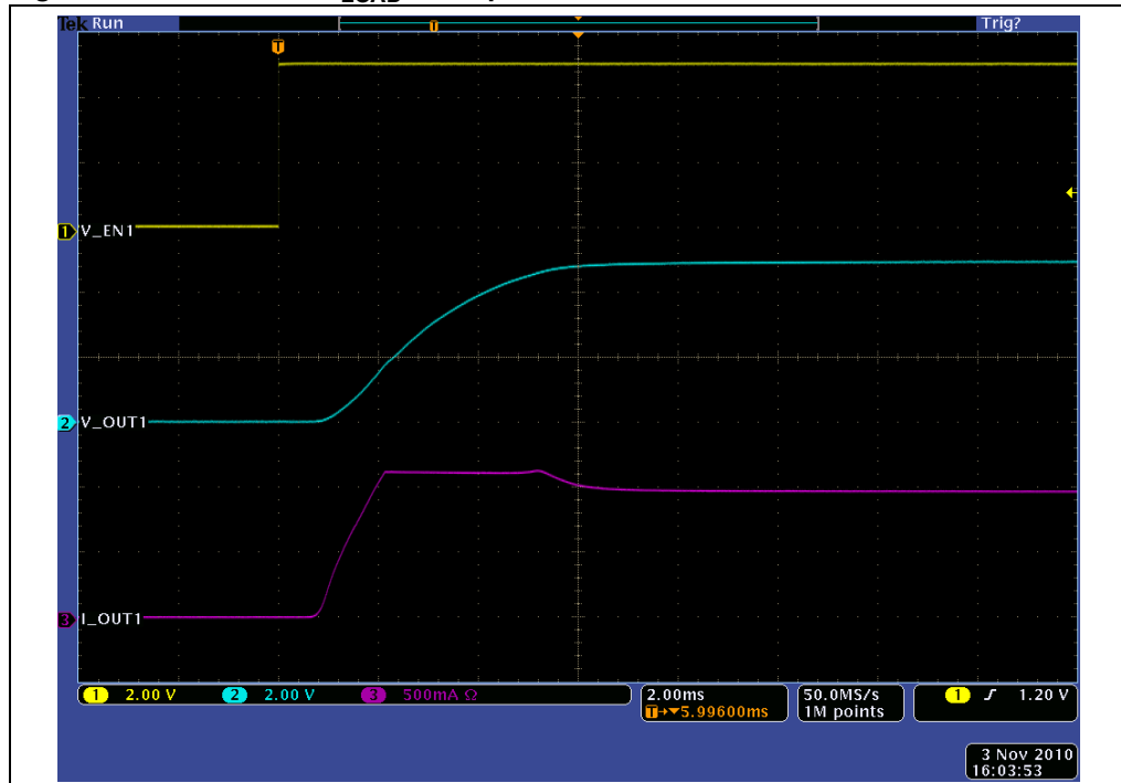
Figure 31. Turn-on for C_{LOAD} = 470 \mu F
