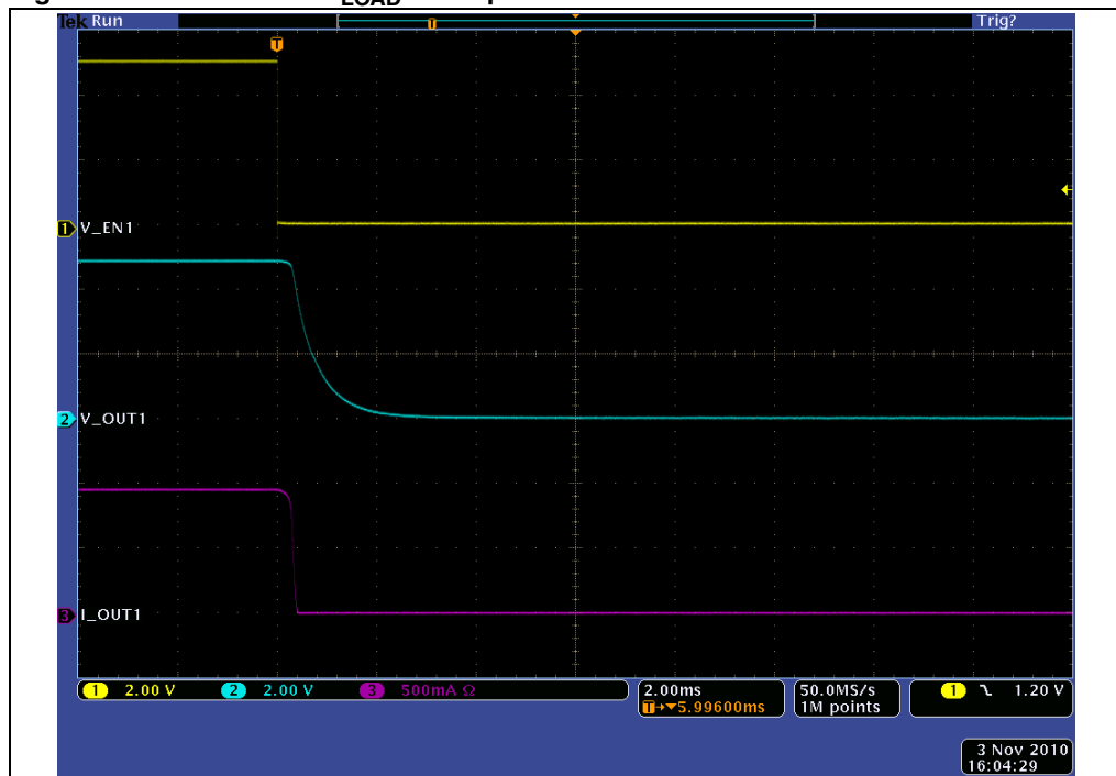
Figure 33. Turn-off for C_{LOAD} = 100 \mu F
