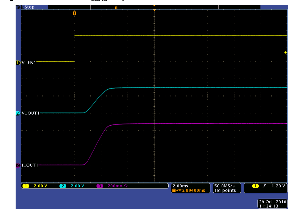
Figure 3. Turn-on for C_{LOAD} = 1\ \mu\text{F}
