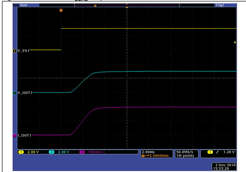
Figure 23. Turn-on for C_{LOAD} = 1\ \mu\text{F}
