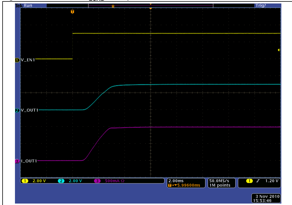
Figure 25. Turn-on for C_{LOAD} = 470 \mu F
