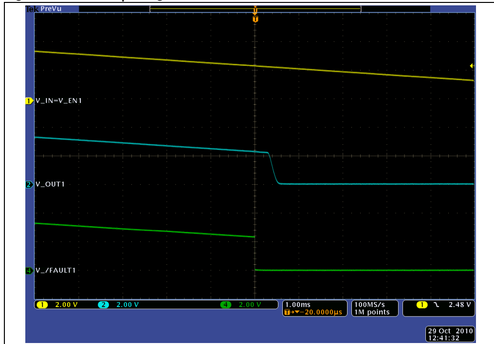
Figure 16. UVLO, V_I falling
