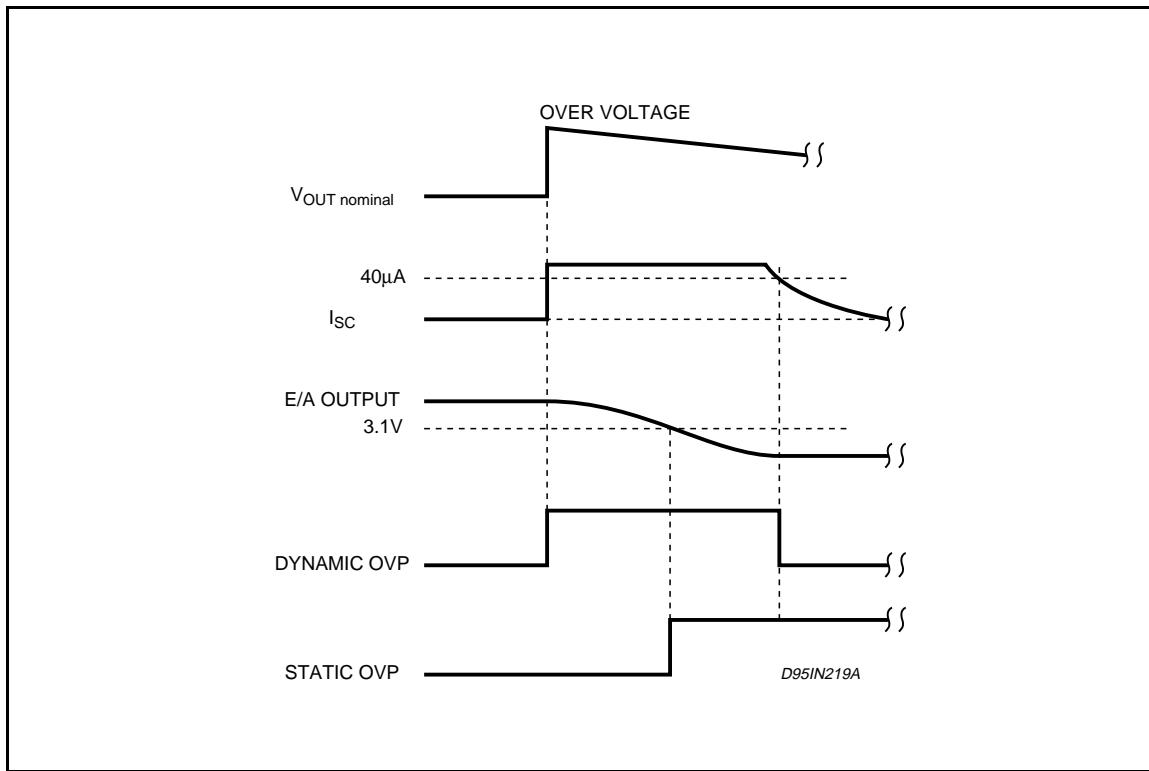
**Figure 2: Overvoltage Protection Circuit**
