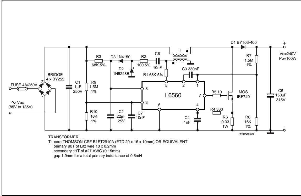
**Figure 4:** Typical Application Circuit (120W)
