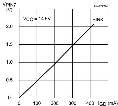
**Figure 11:** Output Saturation Voltage vs. Source Current
