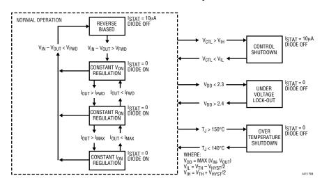
Figure 4. State Transition Diagram
