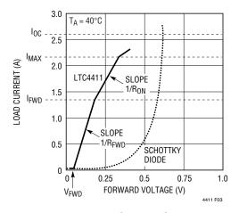
Figure 3. LTC4411 vs Schottky Diode Forward Conduction Characteristics
