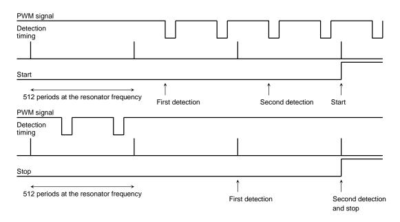
Note: Take sufficient care regarding noise on the PWM signal input pin.
