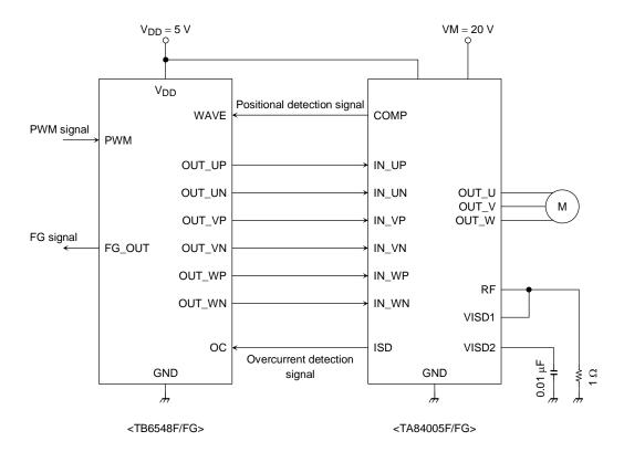
Note 1: Utmost care is necessary in the design of the output, V<sub>CC</sub>, V<sub>M</sub>, and GND lines since the IC may be destroyed by short-circuiting between outputs, air contamination faults, or faults due to improper grounding, or by short-circuiting between contiguous pins.
