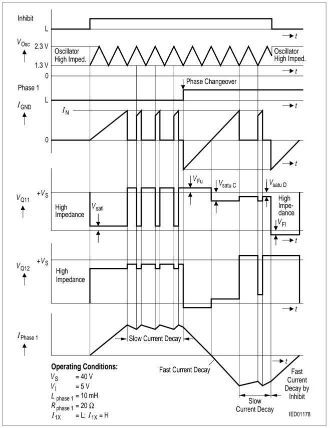
Figure 10 Phase Reversal and Inhibit
