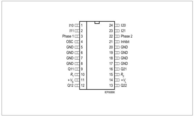
Figure 1 Pin Configuration (top view)
