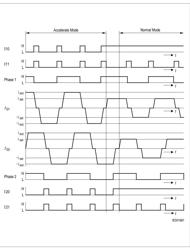
Figure 6 Half-Step Operation
