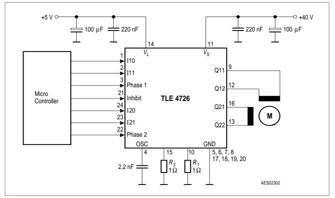
Figure 4 Application Circuit
