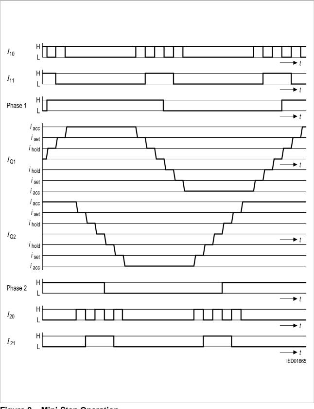
Figure 8 Mini-Step Operation
