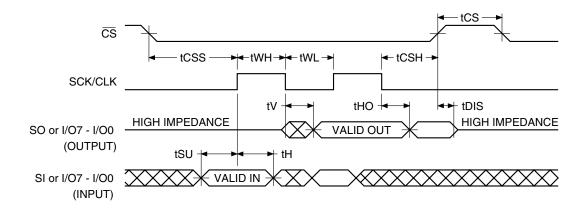
Waveform 2 – Inactive Clock Polarity High and SPI Mode 3
