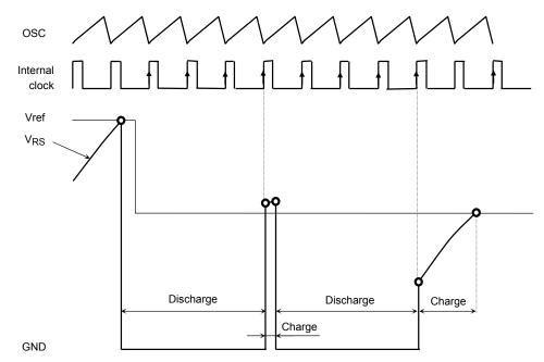
Transition from discharge mode to charge mode
