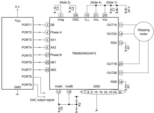
Note 1: A power supply capacitor should be connected between V<sub>CC</sub> and RSA (RSB), and as close as possible to the IC.
