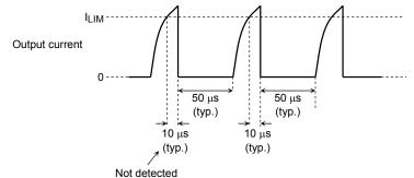
The target specification for the overcurrent limiter value (overcurrent threshold) is 2.5 A (typ.), and varies in a range from approximately 1.5 A to 3.5 A.
