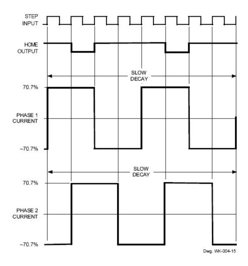
The vector addition of the output currents at any step is 100%.
