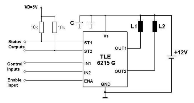
The blocking capacitor C is recommended to avoid critical negative voltage spikes on  $V_{\rm s}$  in case of battery interruption during OFF-commutation.
