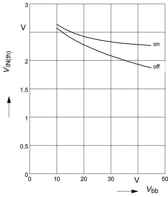
**Typ. input threshold voltage**
