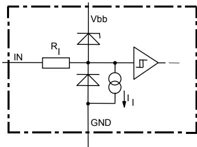
The use of ESD zener diodes as voltage clamp at DC conditions is not recommended
