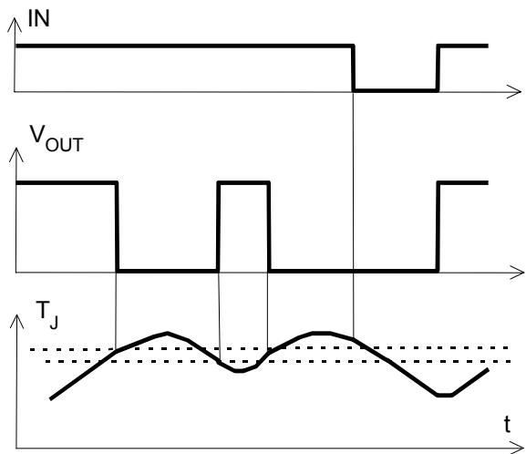
**Figure 3b:** Short circuit in on-state
