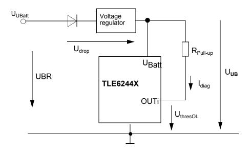
R<sub>Pull-up,max</sub> = (UBR<sub>min</sub> - U<sub>drop,max</sub> - U<sub>thresOL,max</sub>) / I<sub>diag,max</sub>
