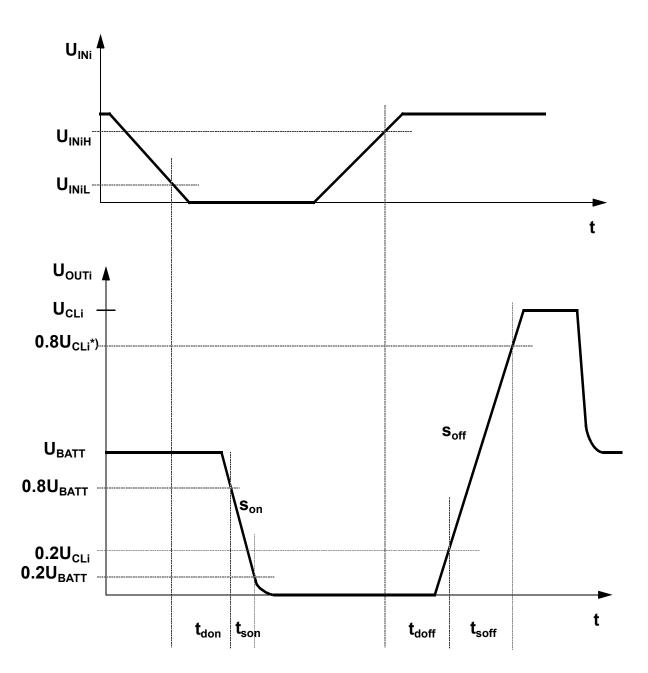
If the output is controlled via SPI the timing starts with the positive slope at SS If the output is controlled by the µsec-bus, the timing starts with the pos. slope of SSY \*) With ohmic load, UCLi = UBatt
