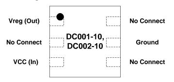
Note: The die attach pad is exposed on the back of this package. NVE recommends that it be connected to the ground pin and the PCB for improved temperature performance.
