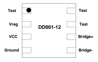
Note: Bridge + and Bridge - should be connected only to the sensor element outputs for ESD and loading reasons. Vreg can supply up to 10 mA at 3.3V ( $330\Omega$  load). Also, all pins labeled "Test" must be floating, *i.e.*, not connected to each other or any other circuit node.
