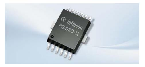
The BTS 500x0-1EGA family consists of single-channel high-side power switches in a green and robust PG-DSO-12-16 package with ON-state resistance (R  $_{DS(on)}$ ) ranging from 5 to 8 m $\Omega$ . The devices offer package, pin and functional (protection and diagnostic) compatibility amongst each other with scaling of R  $_{\mbox{\footnotesize{DS(on)}}}$  and related parameters.
