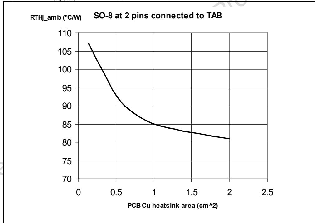
Figure 29. SO-8 thermal impedance junction ambient single pulse
