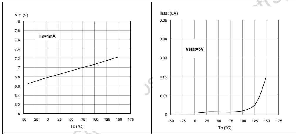
Figure 10. Status leakage current
