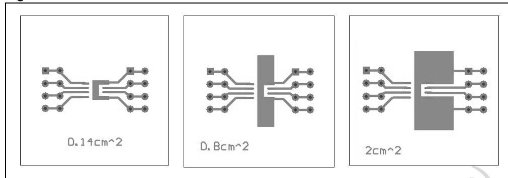
1. Layout condition of  $R_{th}$  and  $Z_{th}$  measurements (PCB FR4 area = 58 mm x 58 mm, PCB thickness = 2 mm, Cu thickness=35  $\mu$ m, Copper areas: 0.14 cm<sup>2</sup>, 0.8 cm<sup>2</sup>, 2 cm<sup>2</sup>).
