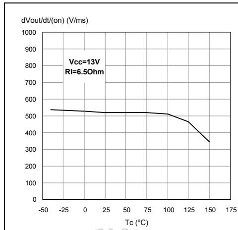
**Figure 22. Turn-off voltage slope (part 1/2)**
