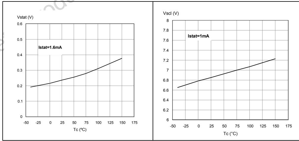
Figure 12. Status clamp voltage
