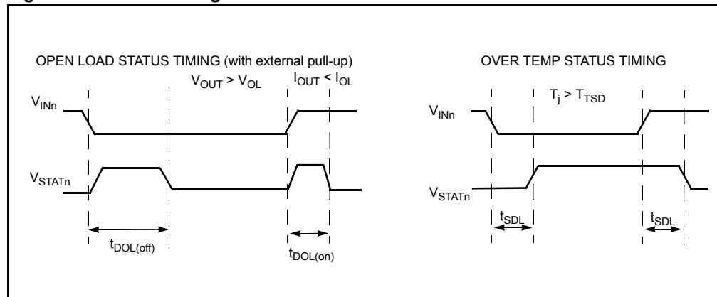
**Figure 5. Switching characteristics**
