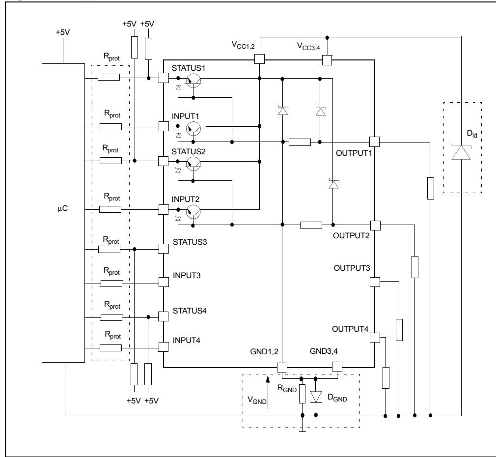
*Note:* Channels 3 and 4 have the same internal circuit as channel 1 and 2.
