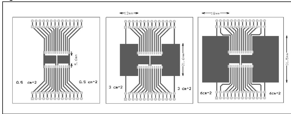
Note: Layout condition of  $R_{th}$  and  $Z_{th}$  measurements (PCB FR4 area = 58mm x 58mm, PCB thickness = 2mm, Cu thickness = 35 $\mu$ m, Copper areas: 0.5 cm $^2$ , 3 cm $^2$ , 6 cm $^2$ ).
