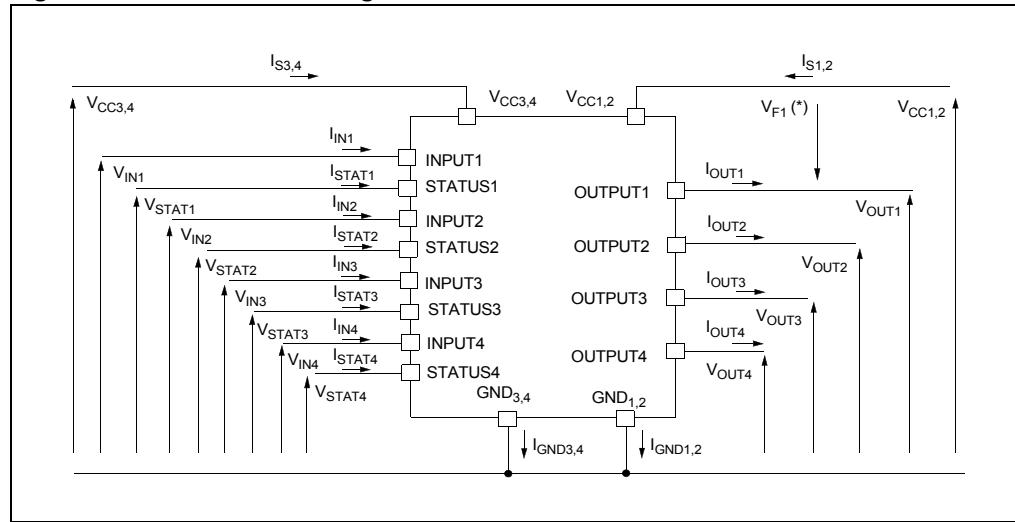
Note:  $V_{Fn} = V_{CCn} - V_{OUTn}$  during reverse battery condition.
