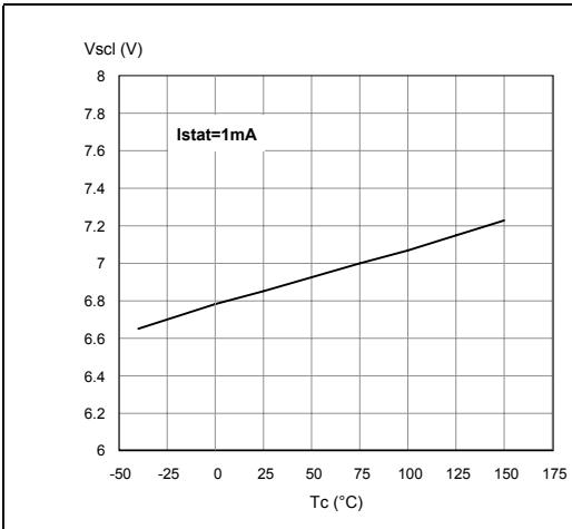
**Figure 22. Open-load on-state detection threshold**
