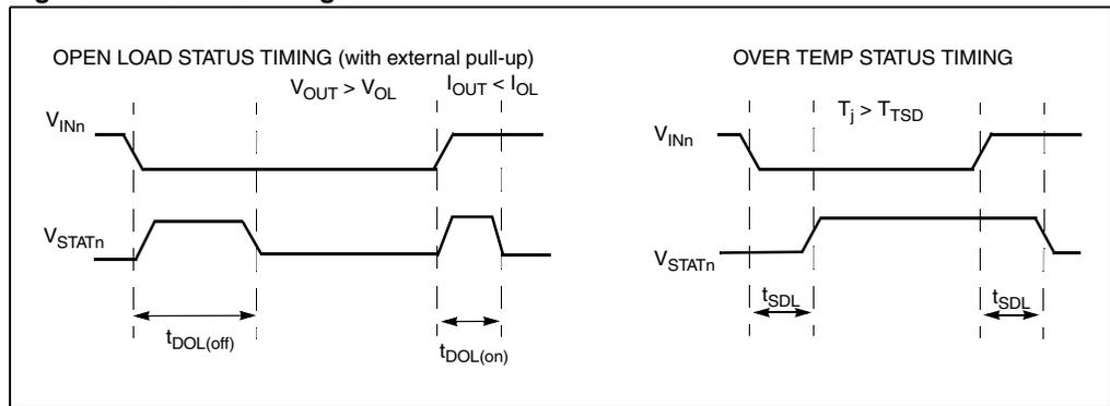
**Figure 5. Switching time waveforms**
