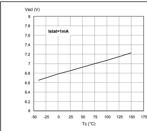
Figure 22. Open-load on-state detection threshold
