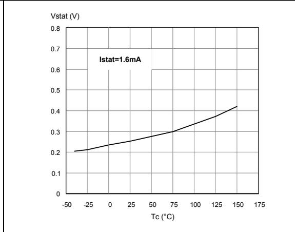
Figure 21. Status clamp voltage
