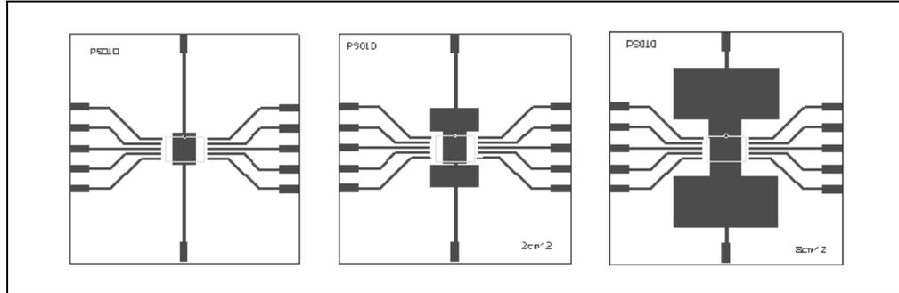
1. Layout condition of  $R_{th}$  and  $Z_{th}$  measurements (PCB FR4 area = 58 mm x 58 mm, PCB thickness = 2 mm, Cu thickness = 35  $\mu$ m, Copper areas: from minimum pad lay-out to 8 cm<sup>2</sup>).
