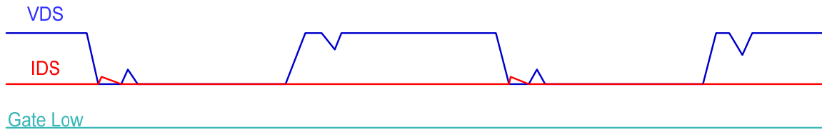
Figure 4: Waveform under MOT protection mode
