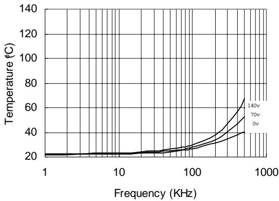
Figure 27. IR21834 vs. Frequency (IRFBC30),
