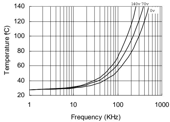
**Figure 37. IR21834s vs. Frequency (IRFPE50),
