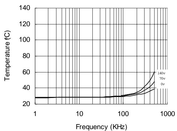
Figure 34. IR21834s vs. Frequency (IRFBC20),
