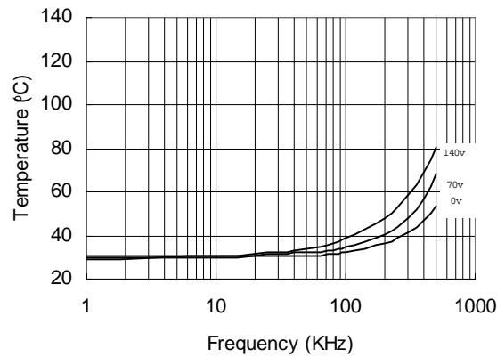
**Figure 35. IR21834s vs. Frequency (IRFBC30),
