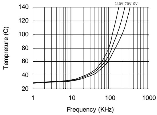
Figure 33. IR2183s vs. Frequency (IRFPE50),
