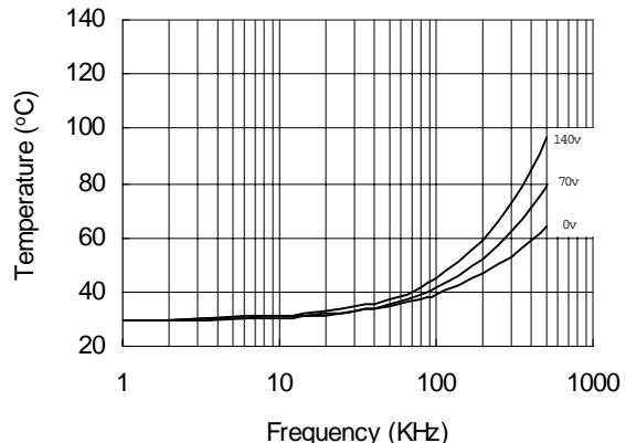
**Figure 36. IR21834s vs. Frequency (IRFBC 40),
