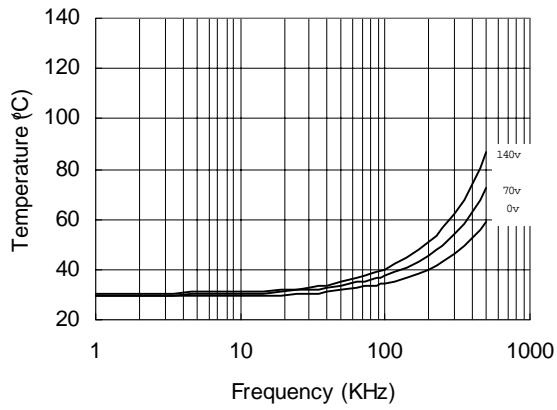
Figure 23. IR2183 vs. Frequency (IRFBC30),
