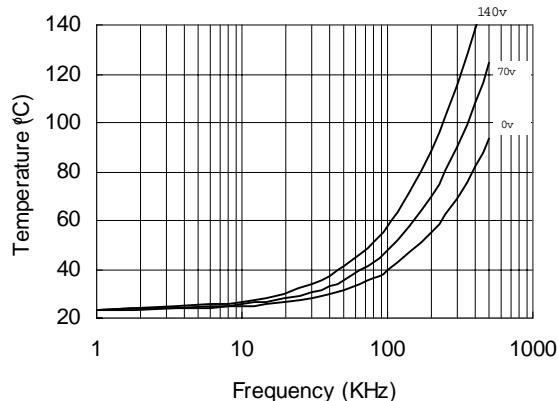
Figure 29. IR21834 vs. Frequency (IRFPE50),
