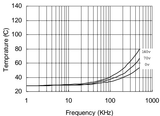
**Figure 22. IR2183 vs. Frequency (IRFBC20),
